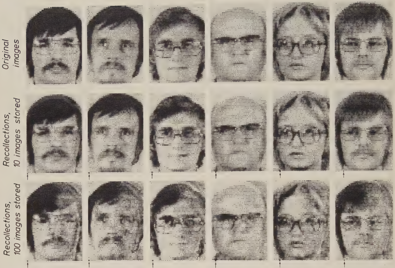
Fig. 2. Autoassociative recall of images when their right half was masked off in the key. First row: Six samples of reference patterns. Second row: Recollections from a memory with ten stored patterns. Third row: Recollections from a memory in which 100 patterns were stored (Arrows: see the text)
